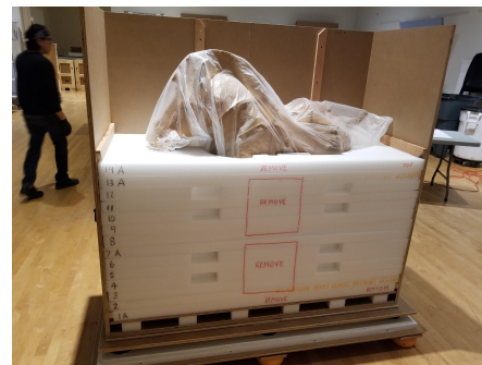
Figure 2. Haniwa Horse , 6th century BCE, LACMA, packing diagram with foam quantity and Haniwa Horse inner box, partially packed. Despite carving the foam to the contours of the sculpture and using vibration-absorbing viscoelastic polymer foam, the artwork broke where it had previously been repaired during transit to the National Gallery of Art in Washington, DC for the exhibition Every Living Thing: Animals in Japanese Art (2019).
